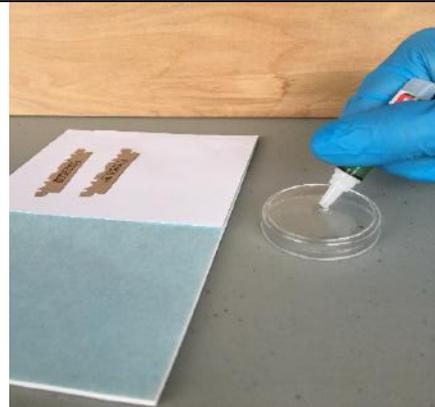
Pipette 5  $\mu\text{L}$  of the super glue onto the blade holder.
