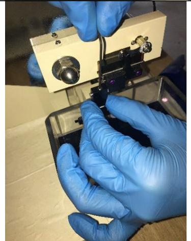
Remove the specimen syringe tube for tissue embedding and loading.
