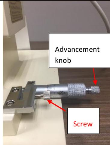
Once manual thickness dial is aligned, tighten the screw underneath.
