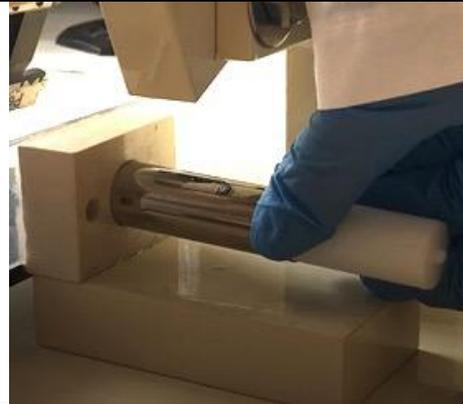
Push the tube as far as it will go into the buffer tray with the tapered end going first. A small stopper knob on the tube will prevent it from sliding all the way into the buffer tray.
