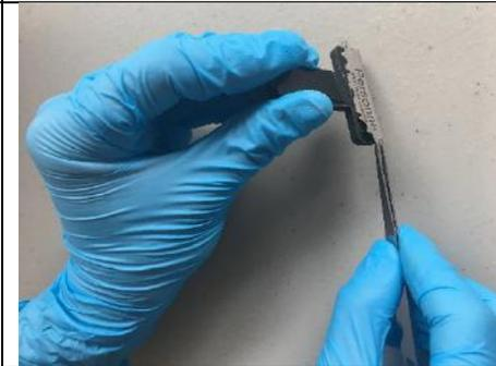
Dip the blade holder into the acetone bath for **5 minutes**. Clean up the residual glue on the blade holder with acetone swabs.
