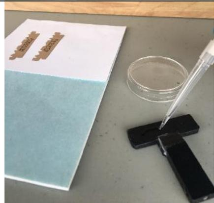
Position the cutting blade onto the blade holder. For the double edge blade, you may notice that along the edge where you cut them, the edges may be curled up. Cut the curled edges of the blade before gluing.
