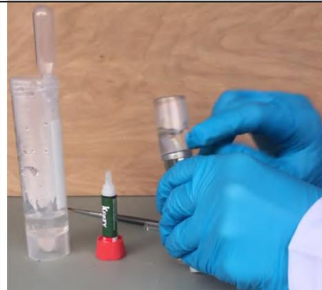
Withdraw the white plunger tube downwards so that the tissue sample enters the metal tube. You can then remove the embedding cap.
