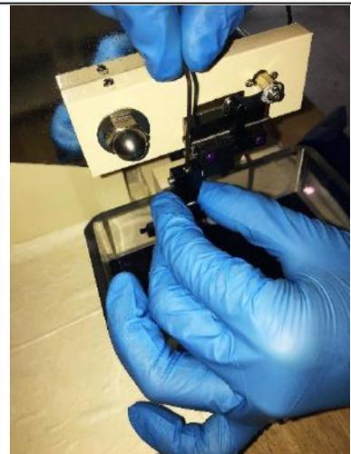
Remove the old cutting blade and dispose of it safely into a sharps container.
