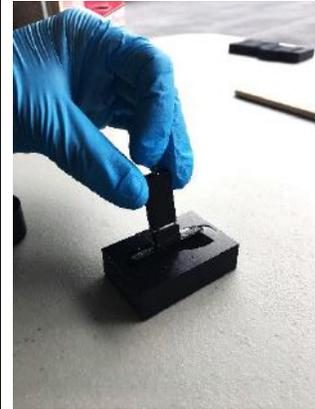
Follow the instructions under “Mounting the Cutting Blade onto the Blade Holder” to install a new cutting blade.
