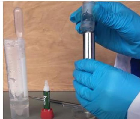
Place the syringe chilling block (should be pre-chilled, see step 1) over the specimen tube to chill the entire sample and help the agarose to solidify. This process usually takes less than a minute, and at most 1.5 minutes.
