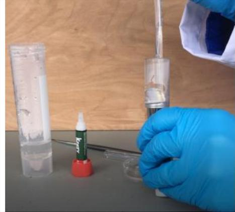
Pipette enough agarose to fully cover the tissue sample. Gently tap on the embedding cap to dispel any air bubbles.
