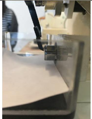
Tighten the set screw on the blade holder in the adjusted position. Make sure that as the screw is tightened, the blade holder does not rotate.
