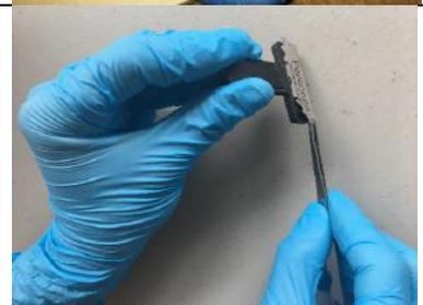
Soak the blade holder in the acetone bath for **5 minutes**. Wipe off any residual glue on the blade holder using a paper towel.
