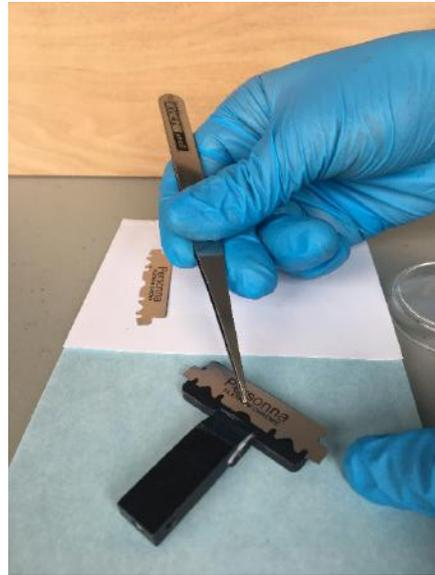
After the glue dries, you are ready to use the blade holder and blade for sectioning.
