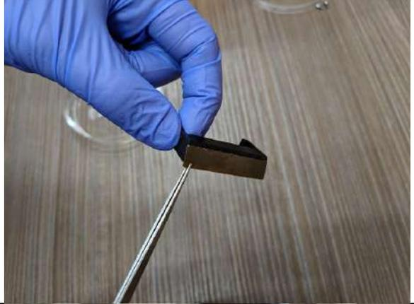
Using an acetone swab, or a paper towel dipped in acetone, rub off any residual glue remaining on the blade-holder.
