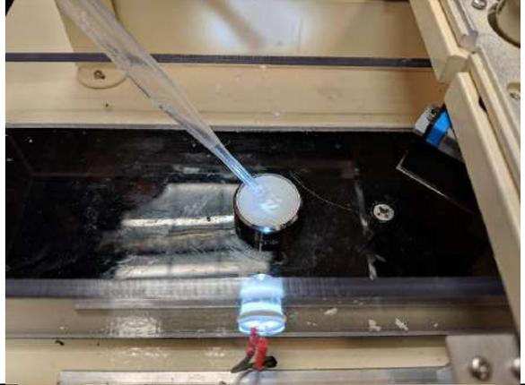
Using forceps, position the tissue onto the specimen tube base and glue your tissue to the base.
