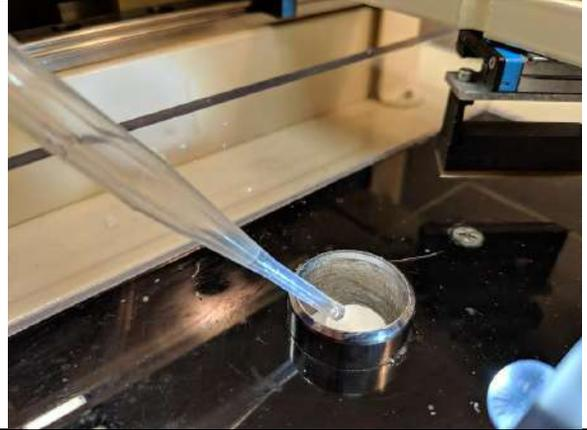
If you want to accelerate the process of the agarose forming a gel, you can pour some chilled buffer solution into the buffer tray (up to the level of the specimen tube, but make sure that no buffer solution mixes with the agarose solution while it is solidifying). Or, place some ice cubes along with buffer solution into the buffer tray.
