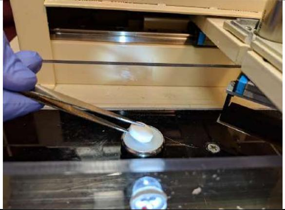
Withdraw the syringe tube downwards so that the tissue sample enters the tube by using the Spec. down switch until the tissue sample is entirely inside the specimen tube.
