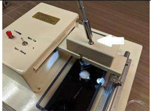
To remove the blade holder from the sliding cutting stage assembly, loosen the two small screws with a small Allen wrench accessed from above, and remove the blade holder from the vibrating head.
