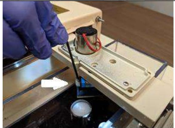
Remove the old cutting blade and dispose of it safely into a sharps container.
