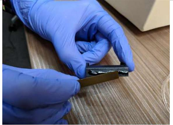
After the glue dries, you are ready to use the blade holder and blade for sectioning.
