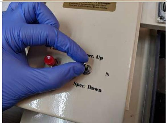
Use the Loading button to move vibrating head up and away from the specimen tube giving you room to work on mounting the tissue.
