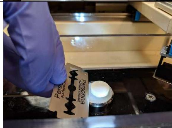
Clean up any debris on the plunger and inside of the syringe tube with acetone swabs or soft brush.
